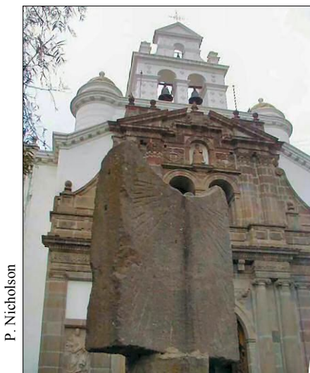
Fig. 7. A vertical dial at the 17 th century church of Guapolo, near Quito, Ecuador. The horizontal gnomon, now missing, would have rested in the channel across the top of the dial.
