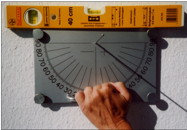
Fig. 5. The pin gnomon of this shadow angle measuring instrument is perpendicular to the instrument face. It has a length of 200 mm and its diameter is 3 mm. The calculation of a wall declination is based on the angle which the pin gnomon's shadow makes with the vertical through its base at a certain time.
