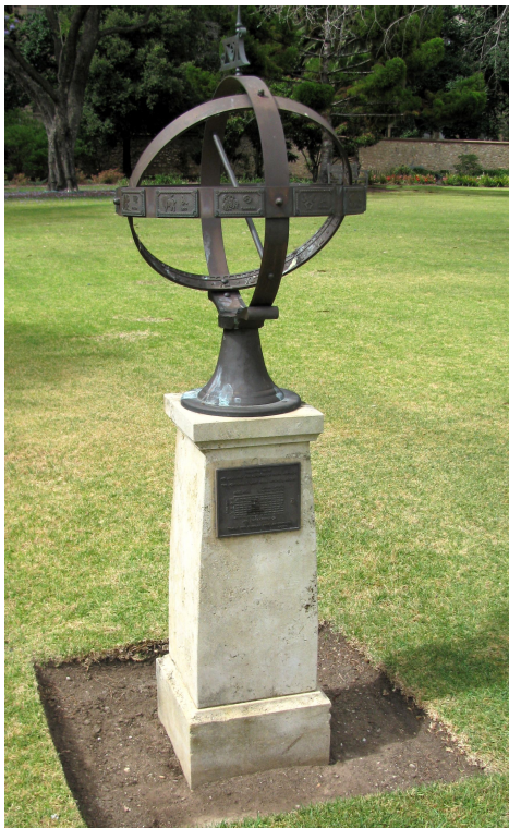
Fig. 5. An earlier design of armillary that has a uniform equatorial ring. Attractive features are the banner on the top and signs of the zodiac on the horizon ring. Sadly the tip and fletching of the gnomon 'arrow' have recently been cut off for safety reasons, but it must be said that the lawns are used for many social functions.
