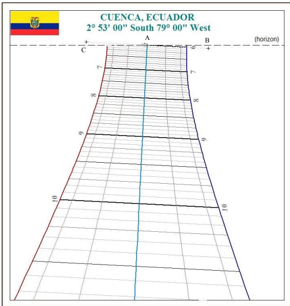
Fig. 9. A design for a direct east dial using ShadowsPro , by François Blateyron.
