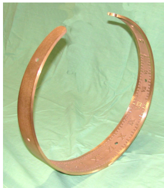
Fig. 8. An hour ring after rolling into shape.
