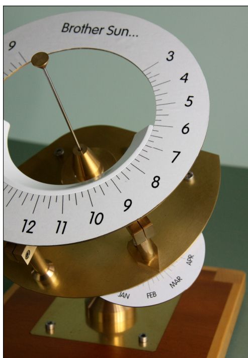
Fig. 7. Month dial fitted to the EoT cam.
