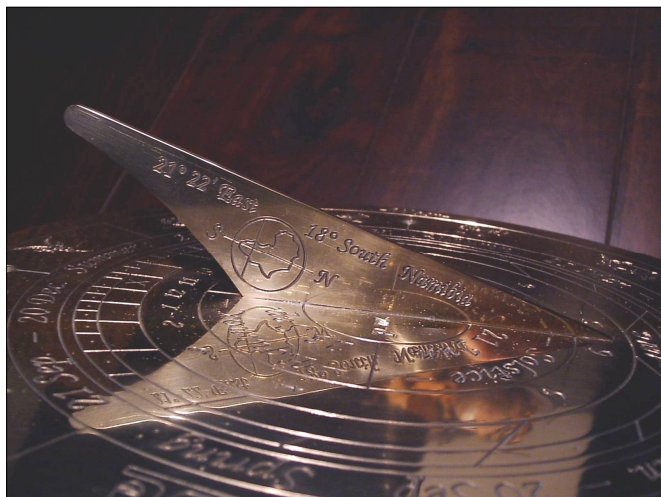
Fig. 1. Horizontal sundial at 18° south. Dial and photo by Henk van der Ham.
