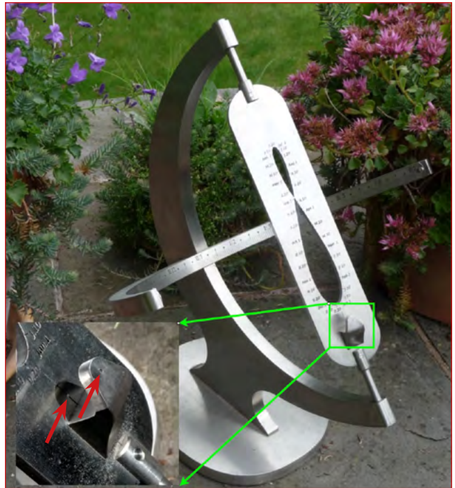
Tony Moss 'Henry Moore' dial - ca 2010 - note the clever arrangement to ensure that the plane of the analemma is perpendicular to the sun's rays
