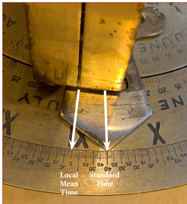
Sol Horometer. The bronze arrow is set for the Longitudinal offset, allowing both local mean time and standard time to be read.
