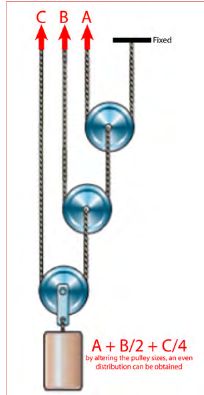
A Pulley Adder
