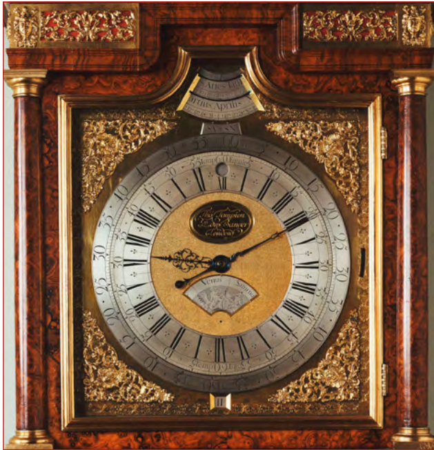
Tompion & Banger - 1703 - Royal Collection. Showing the static Mean Time dial and the rotating Solar Time ring. Note the date is 1st January Julian calendar, being 11th Jan Gregorian, and the difference between the two scales is some 6 1/2 mins - which is about the right value for the Equation on that date.
