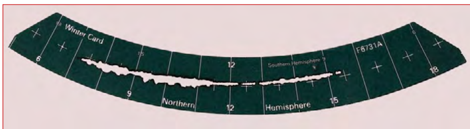
An example of a daily burnt strip. The length of the burnt strip indicated the hours of sunshine during the day In this example, the instrument is not truly set, since the burnt line is not parallel to the central set of crosses.
