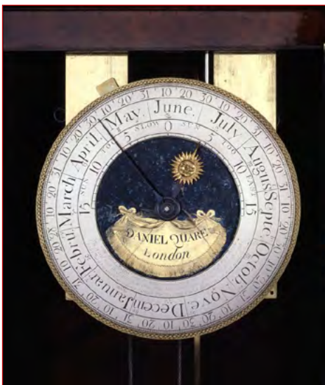
The secondary Equation & Calendar Dial. The Long hand indicates the Date- the Sun indicates the Equation of Time, as Clock Fast or Clock Slow
