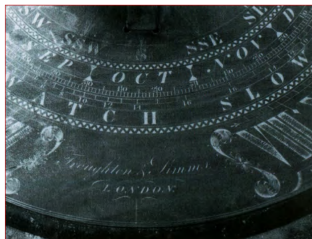
Figure 6: Part of the EoT ring on a late 19 th century dial by Troughton and Simms. The months are written anticlockwise so that the days increase left to right.
