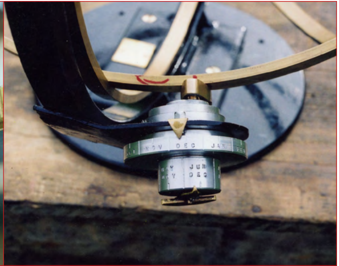
Outer ring and inner cam, showing month graduations - versions 2.
