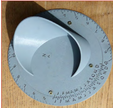
Two of Sawyer-Lelievre Polar Envelope Gnomon Dials a family of dials, such as this, may be 3-D Printed
