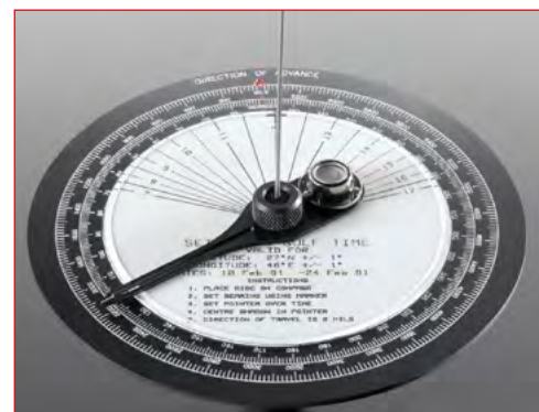
Fig 42 - Howard Sun Compass, pre-marked for mid-February and a Saudi Arabian location in the 1991 Gulf War
