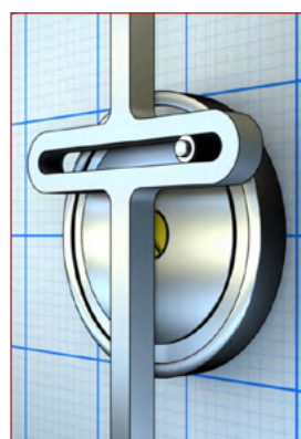
The Tusi Couple. As the Green gear is rotated by the purple arm, the Blue fixed point on the Green gear will move up and down along the Red line with sinusoidal motion.
