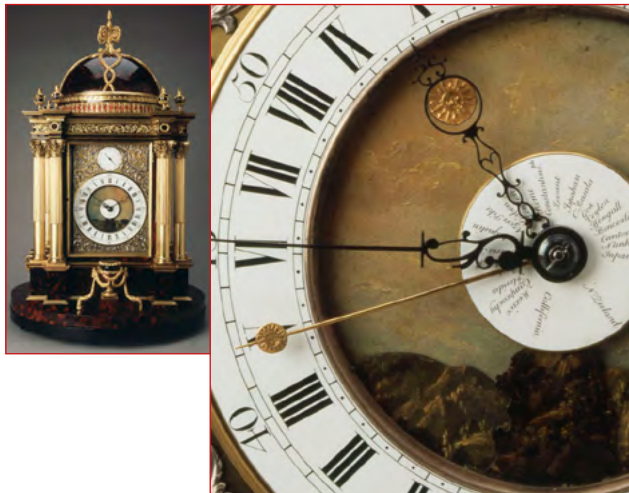
Christopher Pinchbeck - 1768 Note again the golden solar hand, black mean time hand. This photo was taken at 10:45 am, when the background golden sun, corresponds with the hour hand.
