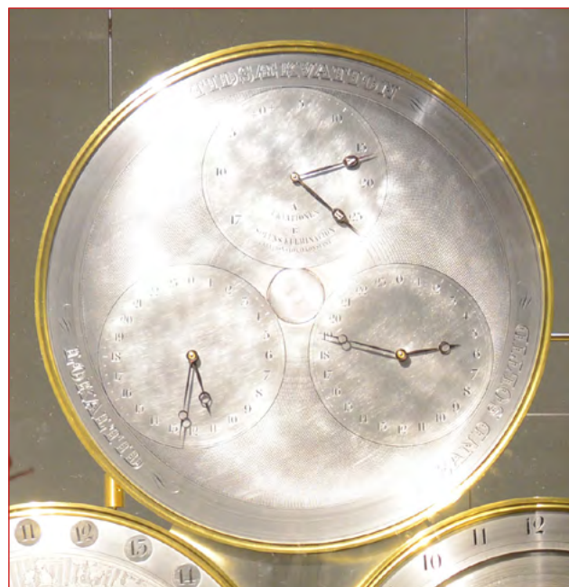
Detail of Equation Clock Face. TOP - (A) Equation of Time & (B) EoT longitude corrected (these hands are fixed 9 mins 47 second apart ; the longitude difference between CET's 15° East and Copenhagen. LEFT Local Mean Time. RIGHT True Solar Time. The clock was not running when this photo was taken (see the vast difference between local and true solar time)
