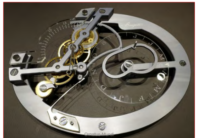
The scythe-shaped cam follower arm is engaged to the kidney cam by the spring at the bottom of the image. This spring is normally disengaged from the follower arm by the small crescent shape in the centre. This rotates to intermittently, releasing the spring and allowing an EoT reading to be taken
