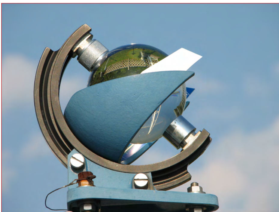
Campbell Stokes Sunshine Recorder. The end of the white back of the cardboard strip sticks out of groves in the instrument.
