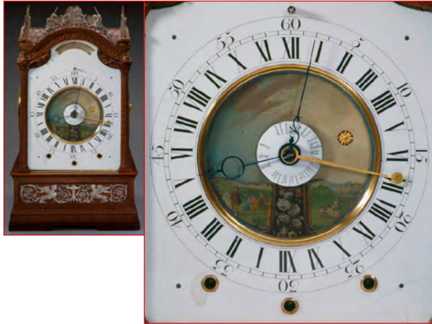
Eardley Norton - 1765 for King George III - Royal Library Windsor. Front Face of Astronomical Clock. Note the 24 hour dial with golden solar hand, black mean time hand and position of the sun in the sky in the background.
