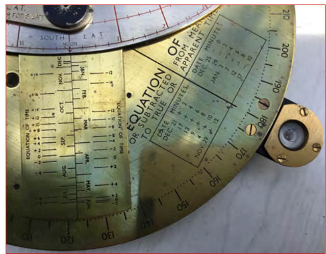
Fig 36 - Date and EoT Scale on Cole Sun Compass: note the EoT scale along the edge of the alidade and also the EoT table covering December and January when the value is changing fastest
