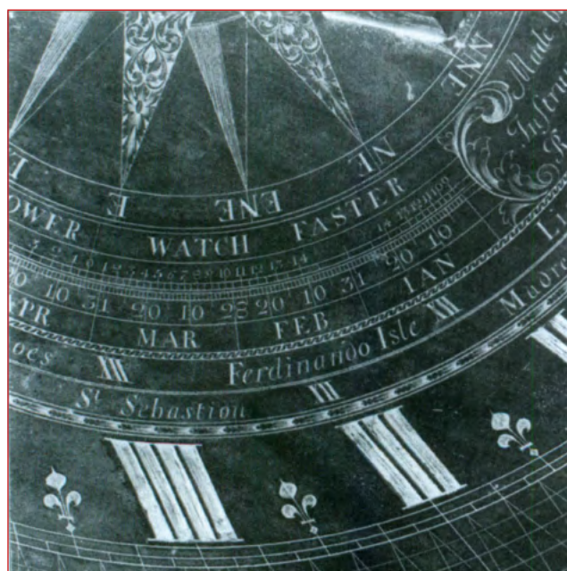
Figure 4: Part of the “Æquation of Natural Days” scale on the Thomas Wright dial at Lacovk Abbey (NT), Wiltshire. Note: the dates increasing right to left and the maximum of 30 Jan in excess of 14 minutes.
