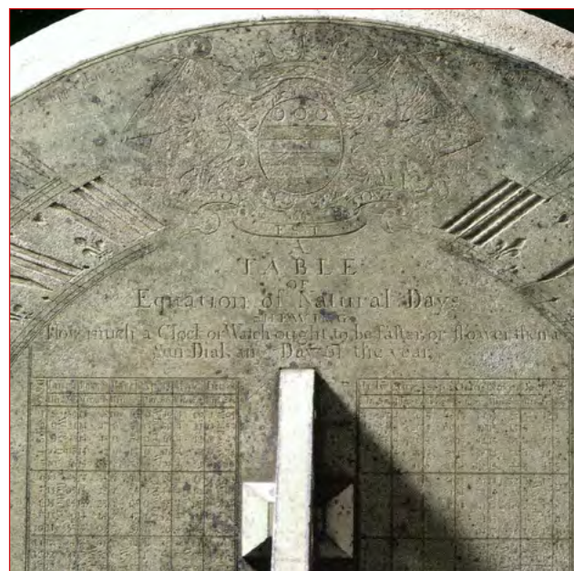
Fig. 2. Part of the EoT table from the Tompion West Park dial, showing the columns for each month of the year. Photo courtesy Sotheby.Åôs
