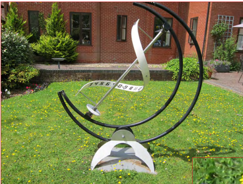
2015 - John Singleton Dial - Stockcross. The spiral mounted on the stainless steel polar axis that can be rotated according to the EoT
