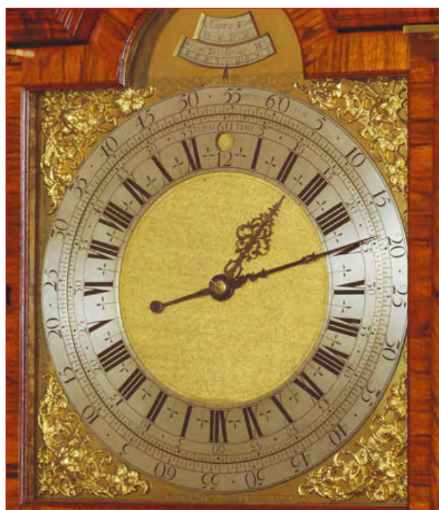
Tompion - 1695 - Morning Room, Clarence House - Note at Noon on the inner Mean Time Ring, the outer Solar Time Ring reads 54 minutes
