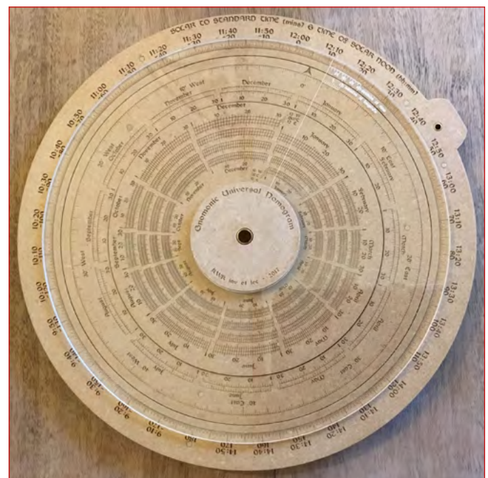
Assembled GUN, as laser engraved and cut.
