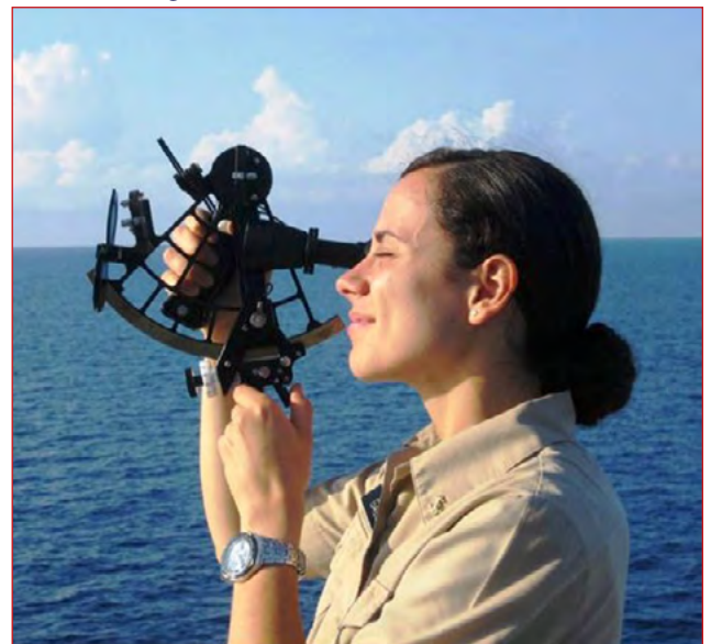
Fig 11 - The Marine Sextant. This works by optically bringing the sun's image of the down towards the horizon. The navigator tracks the sun until it 'bumps' the horizon - that is the moment of solar noon
