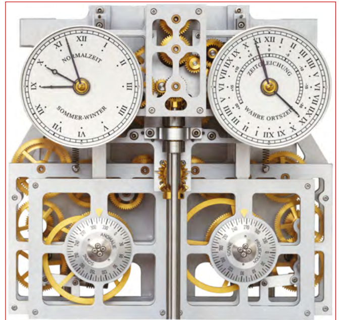
Auxiliary Dials showing summer & winter Civil Time (left) and Solar Time & the Equation of Time (right) with gearing for the Ellipticity effect driven by the anomalistic year gearing (bottom left) and the gearing for the Obliquity effect driven by the tropical year gearing (bottom right)
