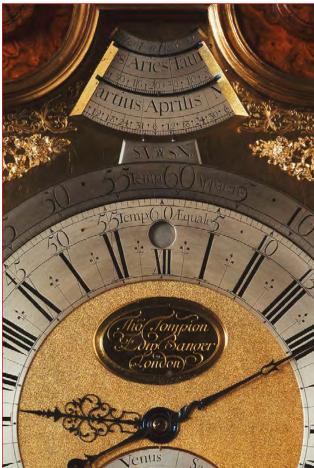
Detail of Tompion & Banger - 1703. Note the Date scale reads 2nd April Julian (SV) and 13th April Gregorian (SN). On this day, the clock gives an EoT of -1 min 20 secs. Tompion's own table (see page 91) for this date in 1683 gives an EoT of 2 mins 4 secs
