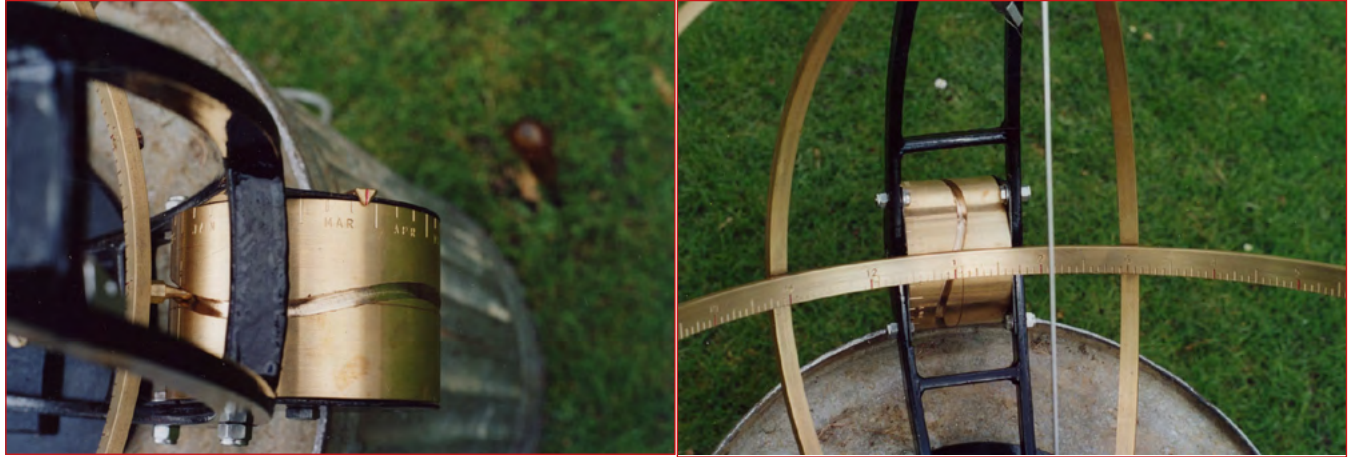
Bill May - 2000 - EoT profile directly drives the equatorial ring of his sundial via a pin which follows the groove cut in the cylinder. The cylinder is marked with the date. The red arrow head shows the month.
