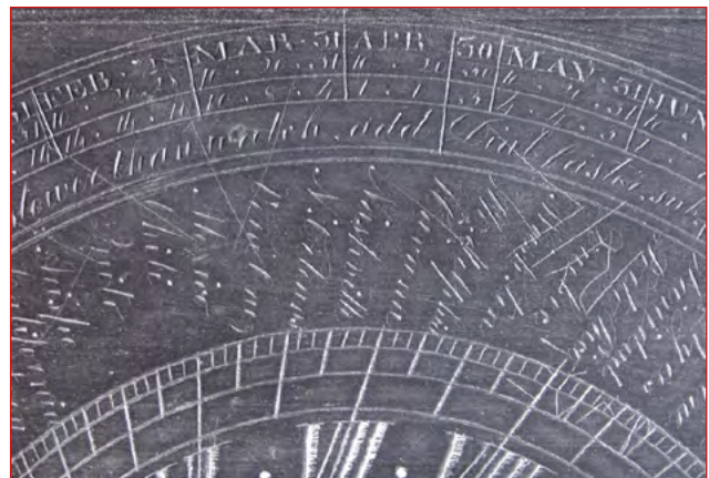
Fig. 13. Part of the EoT ring on a multiple-gnomon slate dial by Richard Melville. This Sussex dial, from relatively late in Melville's career, has the correct value of 4 mins for May 20. Photo: Harriet James
