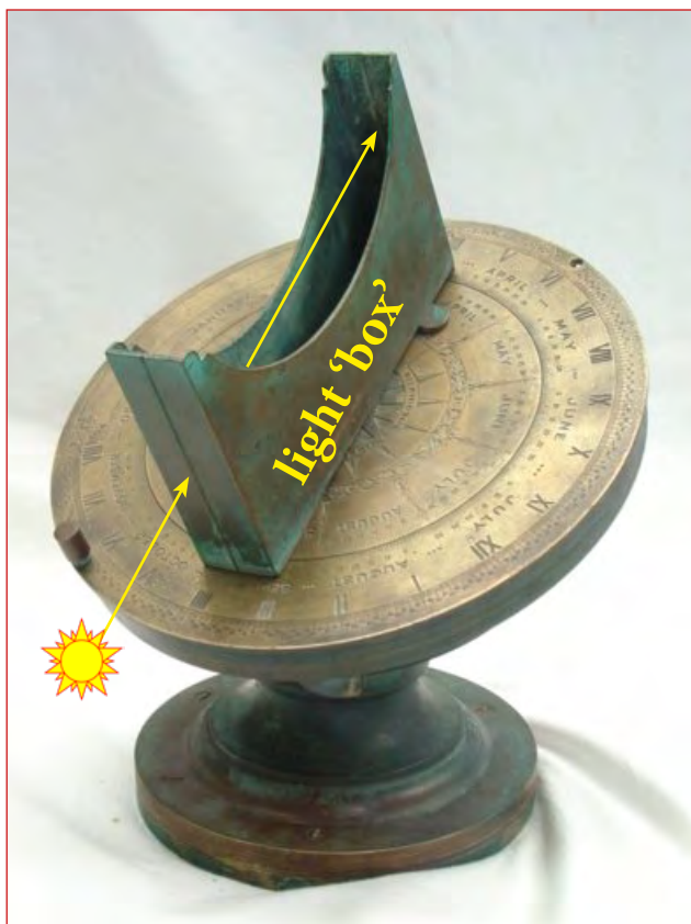
Pilkington & Gibbs' 1914 Sol Horometer has a box-like gnomon with a slit at one end and a 'screen' at the other. The whole box is turn until the sun, shining through the slit hits the screen on the other side of the box.
