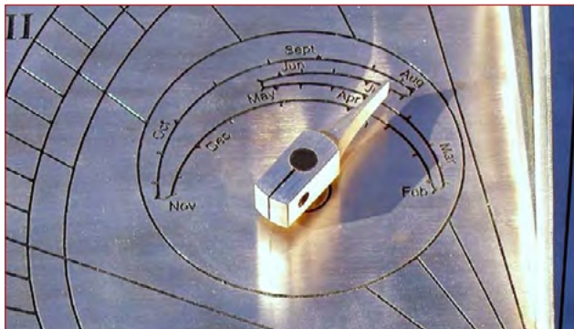
Setting the EoT adjustment on the Sawyer Equant Dial
