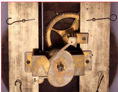
The vertical shaft comes from above driven by the main clock mechanism giving the Date directly and the Equation of Time via the kidney cam.
