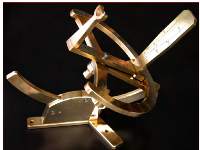
J.D Gard - Aten Heliochronometer - ca 2006 These dials used to be commercially available in bronze or aircraft-grade aluminium
