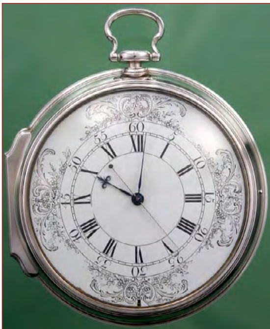
Harrison's H4 1759 Chronometer, whose invention allowed accurate Longitude computation. It took more than 50 years from the invention of the chronometer to be commercially available to all mariners.
