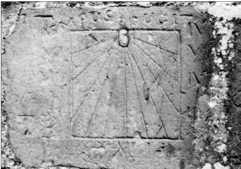
Fig. 1. Londesborough, All Saints. An example of a very early scientific sundial. Note that the hour lines are cut at different angles, narrower near noon and getting wider towards 6am and 6pm. The gnomon is missing but would have been angled away from the dial and aligned with the north celestial pole.
