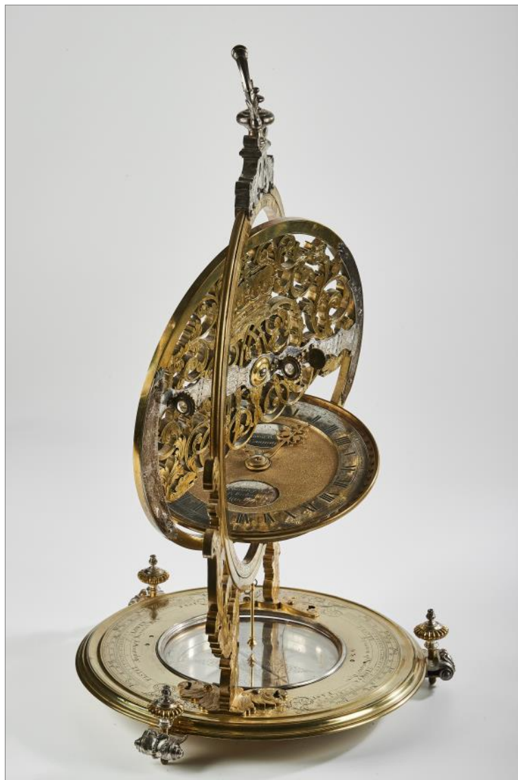
Fig. 8. John Rowley. Mechanical Equinoctial Universal Equatorial Sundial. 1715. © The Peterhof State Museum-Reserve, photo, 2021. Photo: D.G. Iakovlev.
