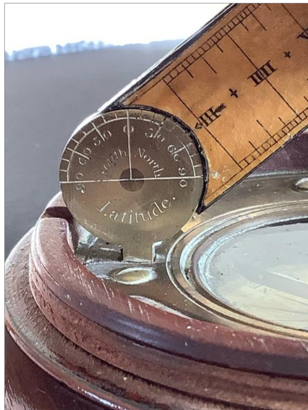
Fig. 6. Close-up of the pivot to set the latitude.
