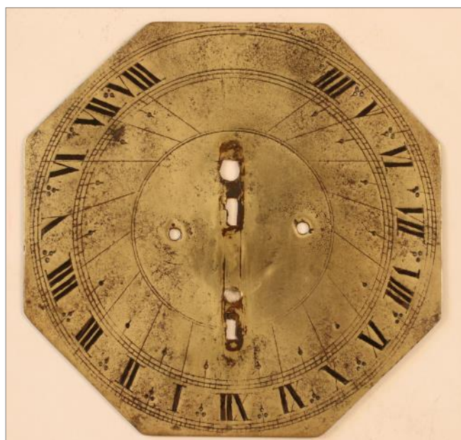
Fig. 4. The cleaned and waxed dial plate.
