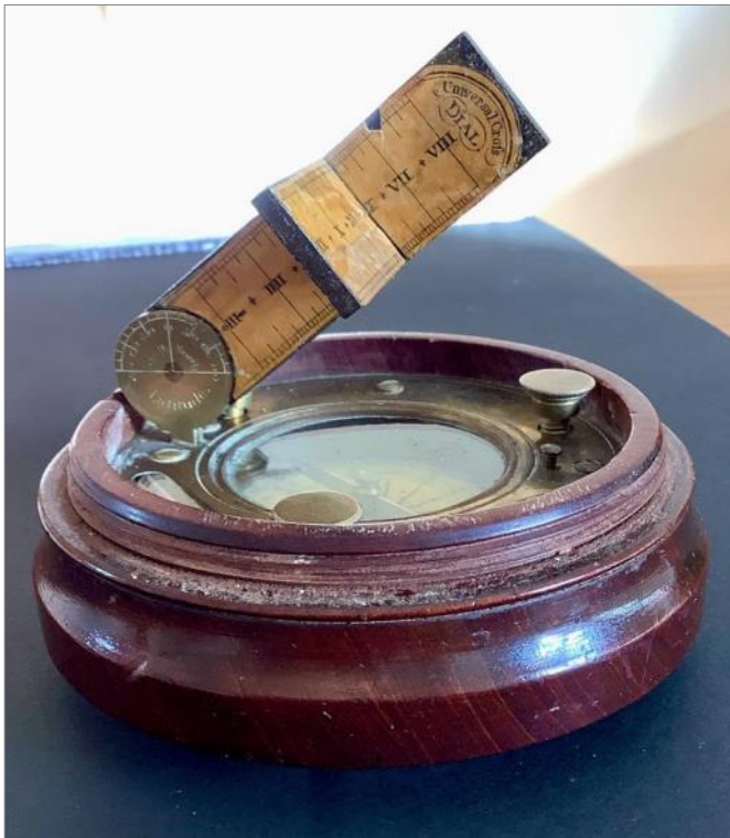
Fig. 7. The cross set up for 50° latitude.
