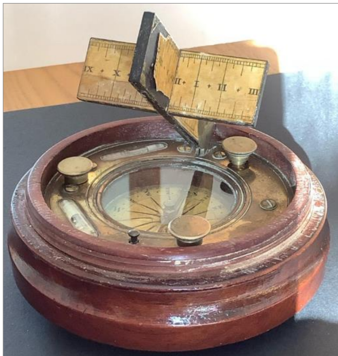
Fig. 4. Hour scales showing 30, 15 and 5 minute divisions.
