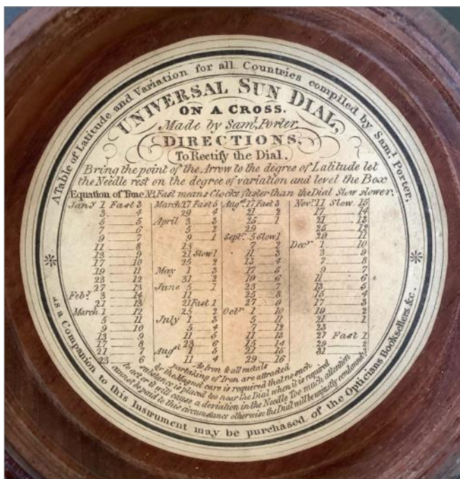
Fig. 5. The inside of the lid with EoT table and instructions for use.
