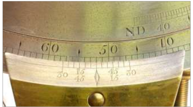
Fig. 6. The vernier scale on the support D, here set to 52°.
