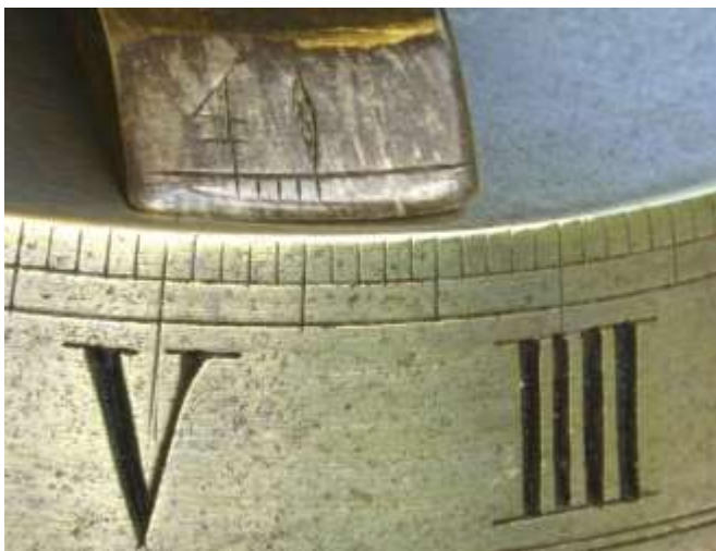
Fig. 5. The vernier scale for the hour readout, divided for every four minutes or one degree.
