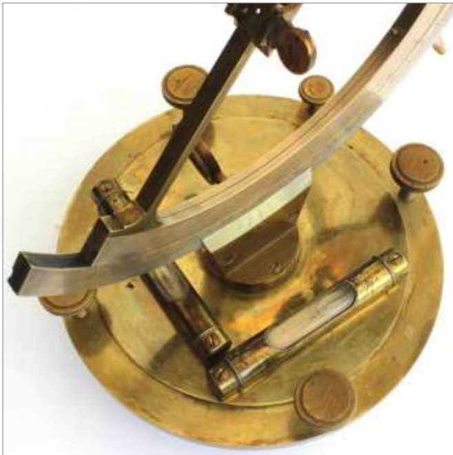
Fig. 3. View from above showing the spirit levels on the rotating base.
