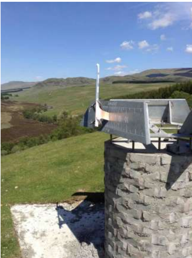
Fig. 7. The dials established in position. There was a brief moment of sunlight and by means of a strip clamped to the gnomon of the south-western face Ben was able to adjust the frame to the right time at 12:00 LST.
