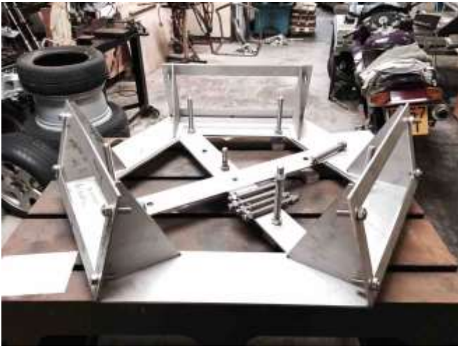
Fig. 6. The stainless steel frame in John Huddlestons workshop. The three oblongs to which the faces are bolted are reclining at an inclination of 71.86^\circ . The base on which the frame rotates slightly can be seen together with the upright levelling bolts.
