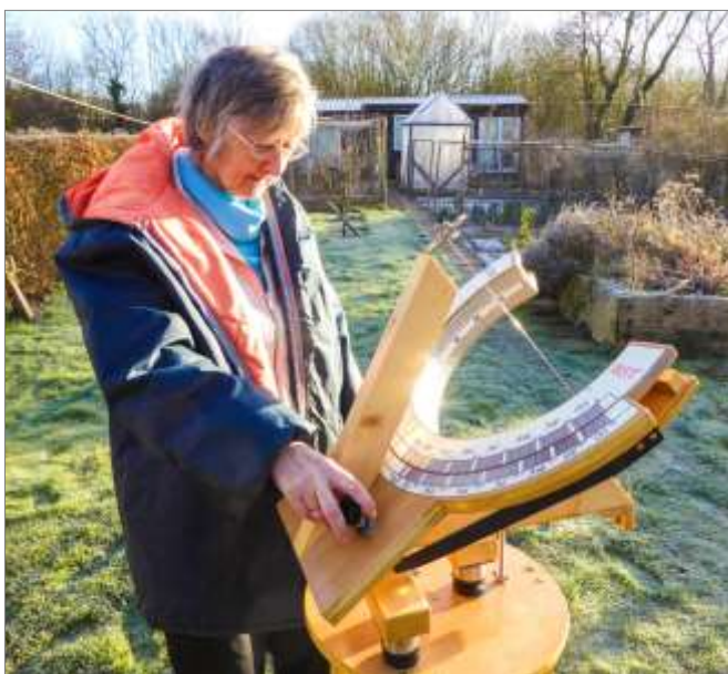
Fig. 9. Setting the EoT correction for the day.
