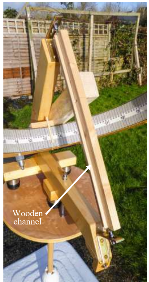
Fig. 10. The gnomon adjustment tool.
