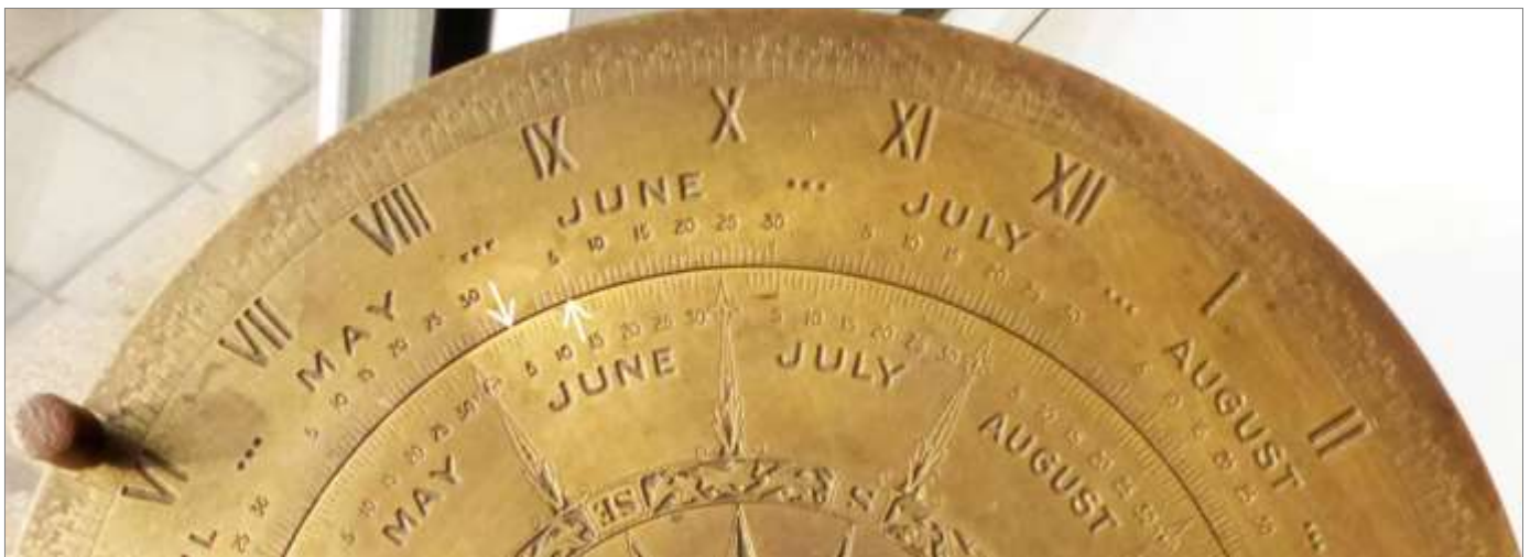
Fig. 13. EoT scale on a Pilkington Sol Horometer (photo: Steve Shaw).
