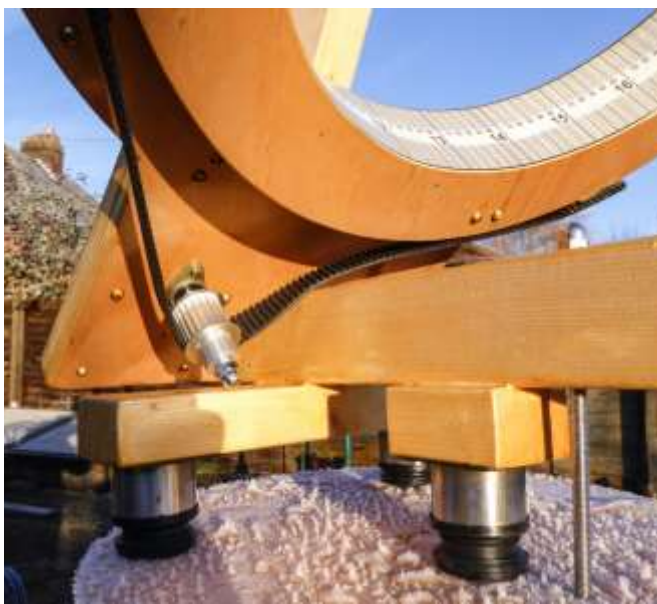
Fig. 8. Mechanism that rotates the timescale arc.
