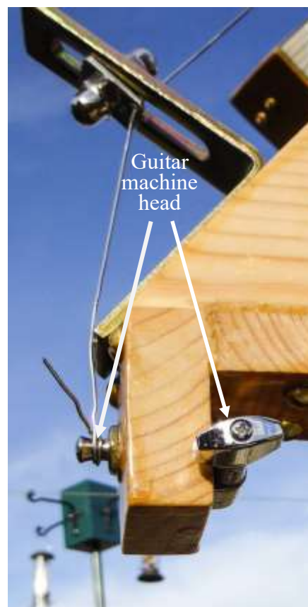
Fig. 6. Guitar machine head used to tension the gnomon.
