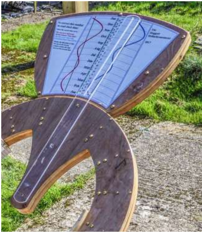
Fig. 11. The EoT correction mechanism of Mark I.
