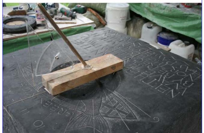
Fig. 7. Setting the gnomon for the St Andrews University Museum Sundial: first, the bronze rod was set in the wax original to form the gnomon and then, after incorporating the gnomon in the mould, preserving its position exactly, the cast was made round the gnomon, replicating its position in the final result.
