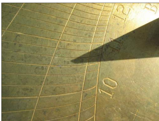
Fig. 11. The complete sundial shown from above. Fig. 12. The time is read from the tip of the shadow.
