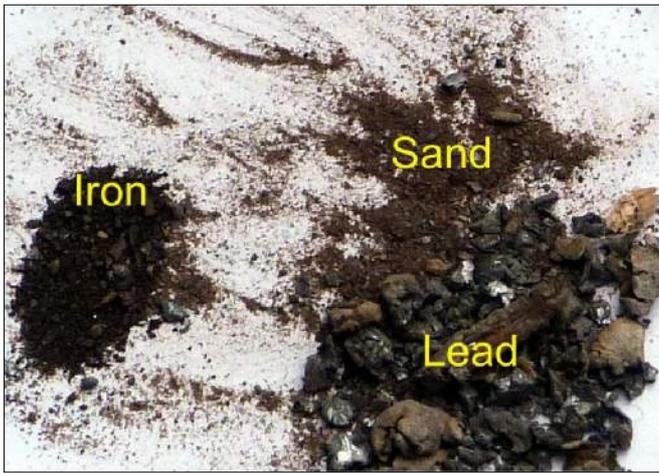
Fig 6. Entire residue recovered from the gnomon slot, separated as iron, sand, and lead particles—the iron was separated by magnet.
