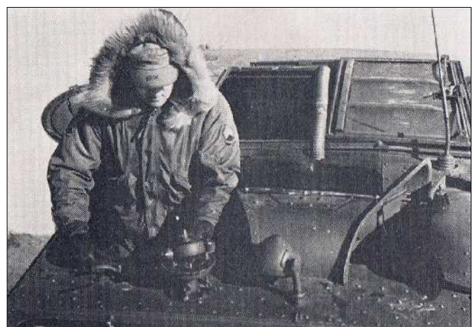
Fig. 3. The Brunson compass mounted on a US Army amphibious cargo carrier.
