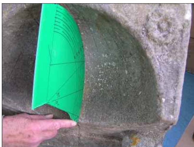
Fig. 4. Testing the sphericity of the surface. Fig. 5. Testing separation of the seasonal lines.
