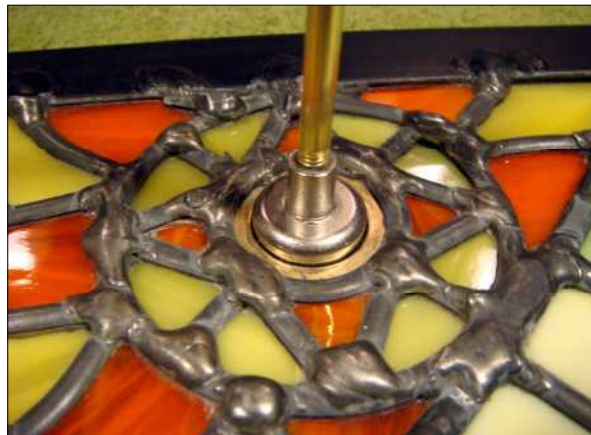
Fig. 5. The mounting magnet fits nicely inside a brass ring and sits on the steel disk.
