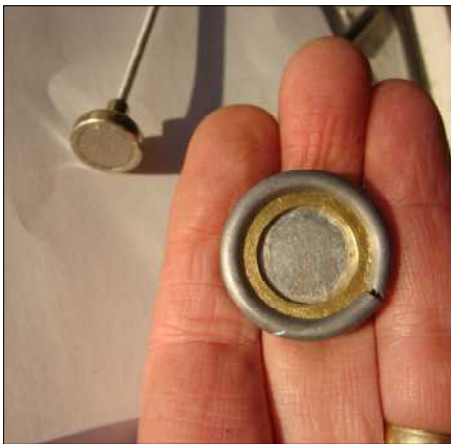
Fig. 4. Steel disk with brass ring surrounded by lead came.
