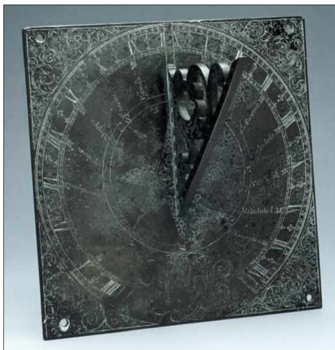
Fig. 6. An early Rowley garden horizontal sundial, dated ca. 1700, with the hour numerals engraved to be read from the outside of the dial, and geographic place names along the hour lines. Courtesy of Oxford Museum of the History of Science.
