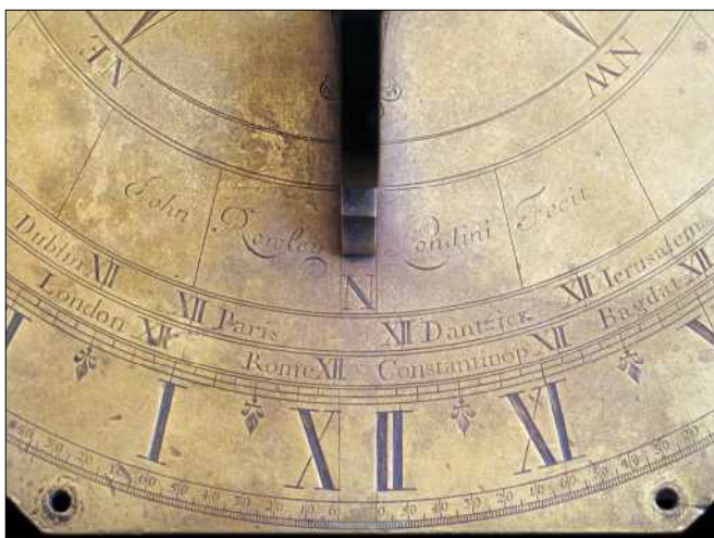
Fig. 5. Lower part of the dial with the detail of John Rowley's florid script signature. Note engraving of the city Dantzick (today's Gdańsk) with the flipped letter 'z' and capital letter 'K'. The two letters are engraved in different style, suggesting that they were cut by a different person.
