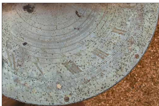
Fig. 7. A section of the Rowley 'geographic' dial at Blenheim Palace, dated 1710, with three rings marked with place names and their local noon times. The Silesian sundial strictly follows this pattern. Note the outward facing hour numerals and inward facing descriptions of the compass rose directions, again like the Silesian sundial.
