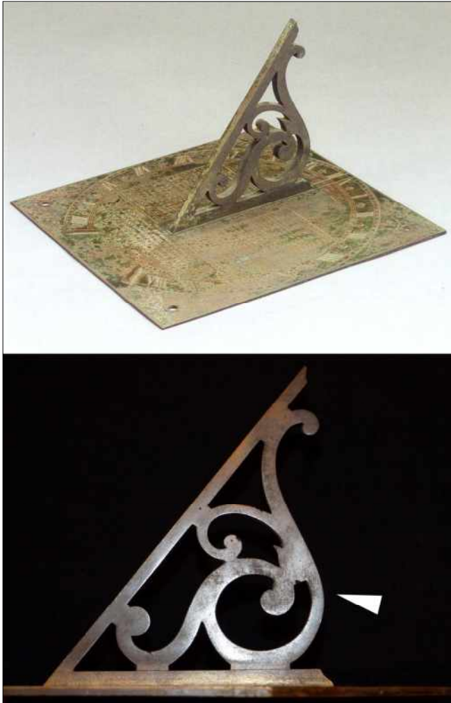
Fig. 10. Comparison of (top) Tho Tompion's signed sundial, dated ca. 1705, and the side view of the gnomon of the Rowley sundial below. The gnomons are very similar but with very minor differences including: shape of the ending profile of the gnomon bars, width of the scrollwork bars with the Rowley's being slightly more lightweight and a shape of the scrollwork in the place marked with an arrow, where the curved lines of Rowley's gnomon are lacking the continuity present in the Tompion example. Tompion sundial image courtesy of Sotheby's.
