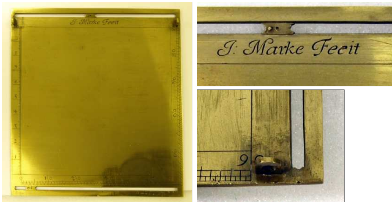
Fig. 2(a) The clinometer side, (b) one of the sights, (c) the signature and one of the sliders.
