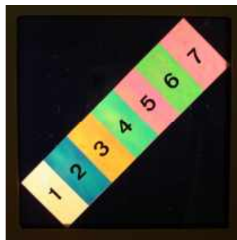
Fig. 2. 1 to 7 superimposed strips of cellophane at 45° between crossed polars.
