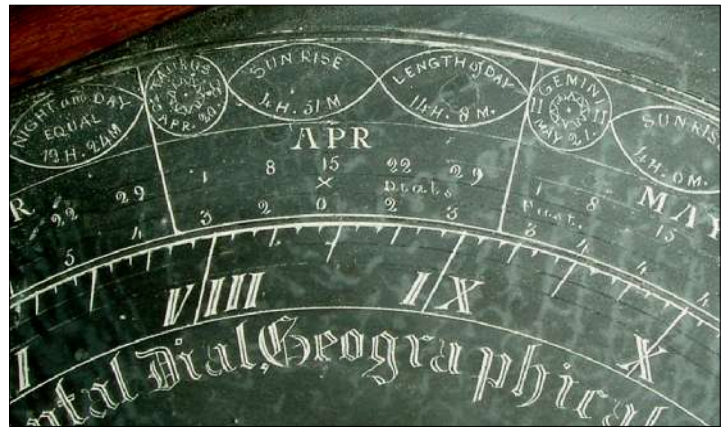
Fig. 6. EoT showing 0 value marked with an ‘x’ on 15 th Apr.
